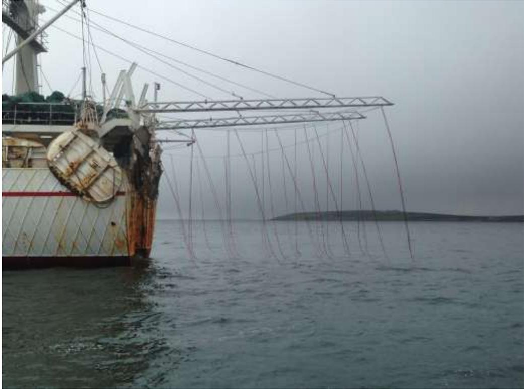
Figure 2. Aerially mounted BSLs attached to booms astern of the vessel
