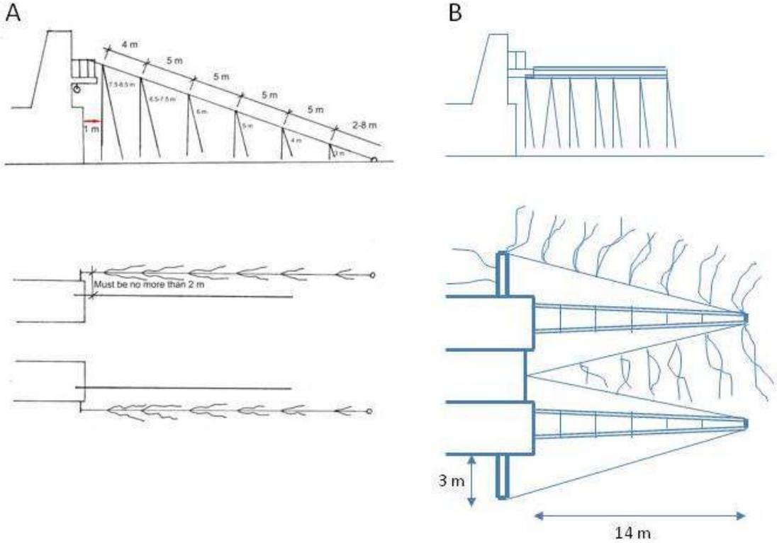
Figure 1. (A) Standard bird scaring lines (BSLs) as currently required by licence and (B) aerially mounted bird scaring lines (BSLs) experimentally trialed in this report. Note streamers were attached to both sides but in this diagram only the starboard streamers are shown.
